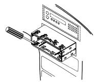
5. Slide the bracket into the console until it clicks into place.
